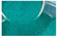
Utilizing a colored carbon fiber compound instead of a glass fiber filled compound, affords a mechanical designer the potential to match or improve the strength and stiffness of a part while reducing the part's weight. The designer has the potential to increase the strength and stiffness of a part without increasing the part's weight. This ability can become a game changer in applications where colored components are at their maximum limits with glass fiber filled compounds.
