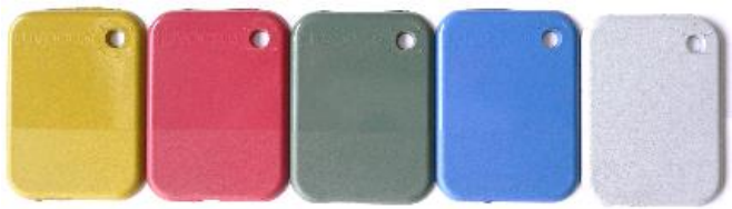
Colored carbon fiber compounds based on PA 66
